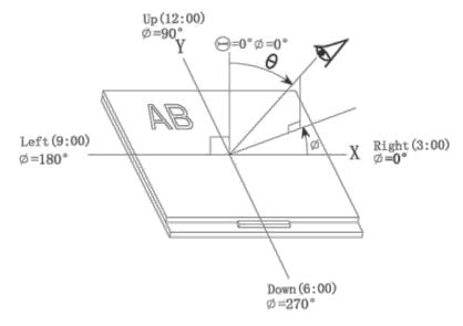
Note 4: Definition of contrast ratio Contrast measurements shall be made at viewing angle of  $\Theta$ = 0 and at the center of the LCD surface.Luminance 15 shall be measured with all pixels in the view field Victronix Display Co., Limited Tel:86-755-33265935 Email:sales@victronix-tech.com
