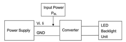
Note 3: The "LED life time" is defined as the module brightness decrease to 50% original brightness at Ta=25°C and If =80mA. The LED lifetime could be decreased if operating If is larger than 80mA. Note 4: LED light bar circuit:
